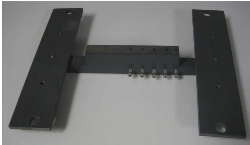
Figure 2.5: Thermocouple Holder (Bottom View) (Zantout, 2009)
