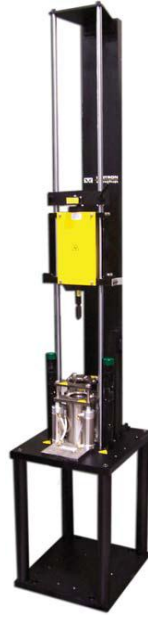
Figure 2.8: Instron 8200 Impact Tester (Dynatup, 2010)
